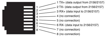
Figure 4. CopperLink Ethernet Extender 10/100Base-T RJ-45 Connector Pinout.
